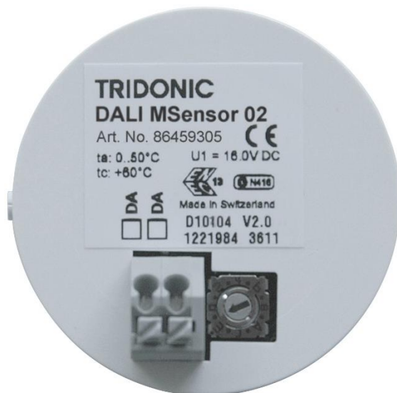
Figure 176: Set MSensor 02 5DPI 41 group dial to position 'F'.
