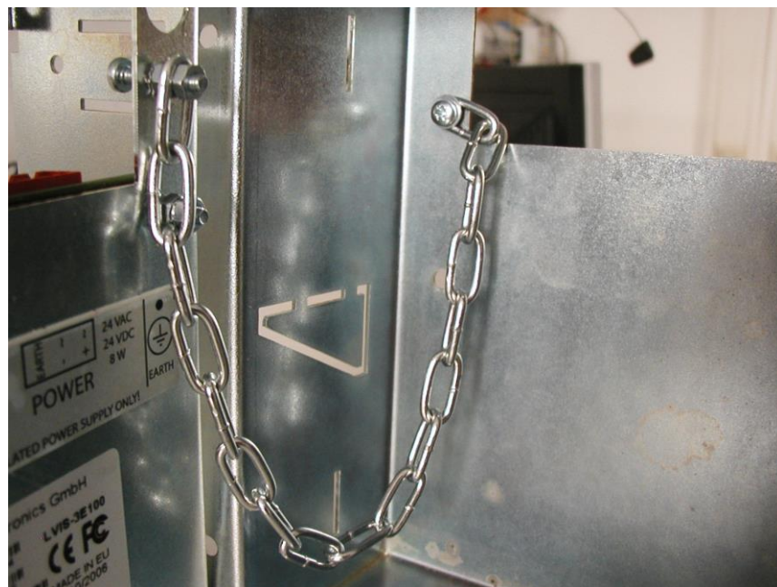
Figure 1: Connecting L-VIS to the wall mount frame.
