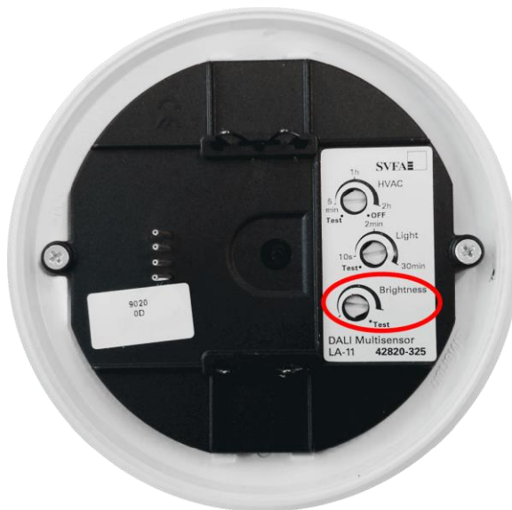
Figure 180: Ensure position of Brightness dial is not set to Test.
